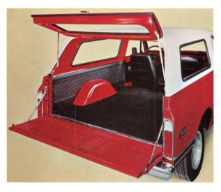
Lockable lift gate on hard top opens up for easy, convenient rear loading. Telescoping supports keep lift gate safely in open position.
